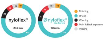
Overall 20% faster plate processing possible when using nyloflex® eco plates (in direct comparison to standard nyloflex® FAC)
