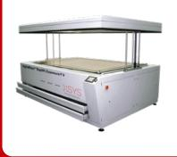
The nyloflex® Toplift Exposure F V is equipped with a glass exposure bed for back and main exposure without turning the plate around. The toplift design offers an optimal accessibility from all sides. The unit includes a digital display to record the operating hours and a new generation of electronic ballasts, which doubles lamp life compared to conventional ballasts.
