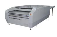
Fully automated system for wash out, rinsing, after cleaning and pre-drying of mid and large formats. Individually adjustable parameters for transport speed and brush height. Optimal washout result through integrated solid content measurement device. Washout solvent is controlled to ensure a constant temperature. One-person operation. Escaping vapours are reliably exhausted. Low noise level during the process.
