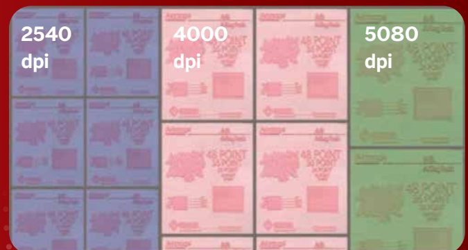
Flexo plate with different jobs at different resolutions
