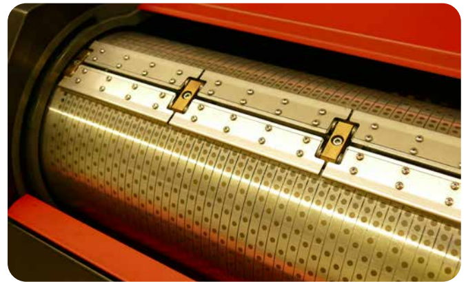
Hybrid drum for Flexo and Steel back Letterpress plates
