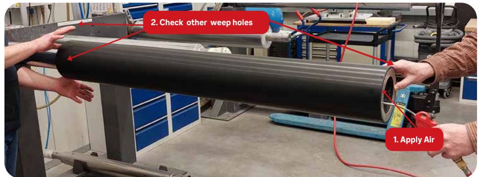
Fig. 2: Weep hole maintenance
