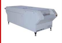
The compact, tankless flowline system provides water washout, drying and post exposure all in-line. The proven and easily adjustable plush system provides optimum washout results while the touchscreen offers easy operation, including control of the water temperature and flow speed control. Includes adhesive carrier plate for foil based plates and magnetic carrier plate for metal based plates.
