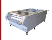
A tankless flowline system, offering water washout, drying and post exposure all in-line. A touch screen display offers easy operation, including control of the water temperature and flow speed. The proven ,plush' system that is easily adjustable, provides optimum washout results. Includes automatically lowering squeegee roll, adhesive carrier plate for foil based plates and magnetic carrier plate for metal based plates.
