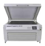
Premium quality system for main and post exposure as well as drying of nyloprint® printing plates with integrated chiller. It includes four drawers and 20 memory programs for main and post exposure. Operation of each tube is monitored and operating hours of tubes are recorded.
