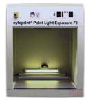
Table top point light exposure unit with a metalhalide lamp. Ideal for high quality pad printing applications. Includes automatically controlled front door panels for optimum UV-protection, a yellow tube to illuminate the working surface and an operating panel with digital display to set up exposure times.
